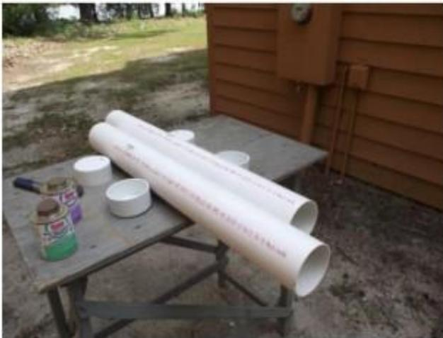
Note that this is 4" diameter thin-wall drain pipe. It is cheaper and lighter than schedule 40. The 4" caps shown are sold in the same section of most building product stores.
