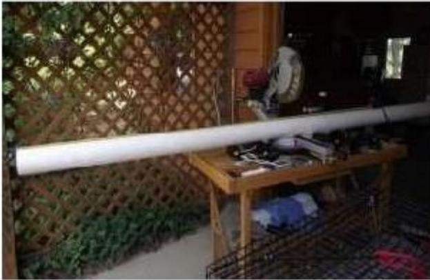
PVC drain or sewer pipe comes in 10 foot lengths. Cut one 33.5 inch piece for each Tidal Tumbler. None are required for a Rough Rider. You can cut the pipe with a compound miter saw, jigsaw, circular saw, or hand saw. Note that this is 4" diameter thin-wall drainpipe. It is cheaper and lighter than schedule 40 PVC pipe. The 4" end caps shown are sold in the same section of most building product stores.
