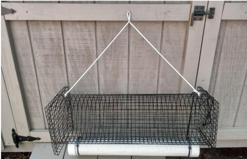
For the Tidal Tumbler only, attach the PVC tube along the overlap seam. Use a 24 inch cable tie at each end just inside of the end cap to secure the PVC tube to the wire cylinder. Cut off the excess cable tie once secured. Use a 5 foot piece of crab pot line to create a harness which is attached opposite from the PVC float. Use 2 pig rings for the loop at the apex and to attach each end.
