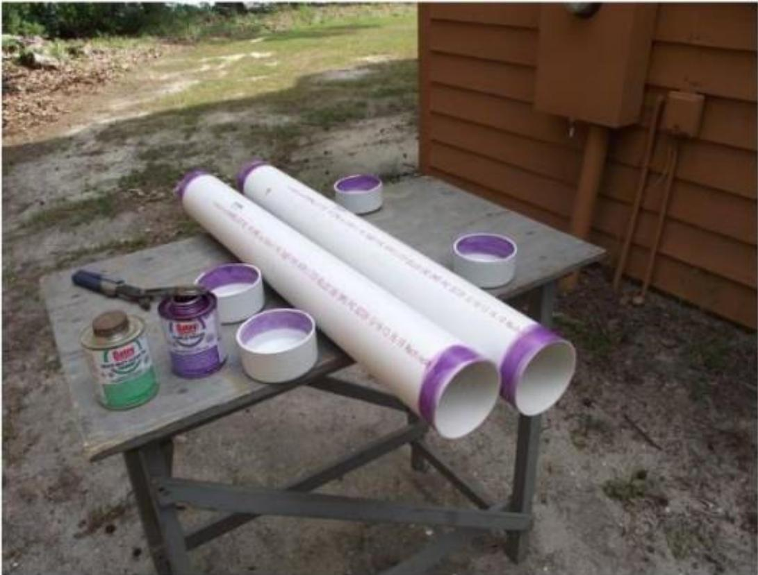
Prime the pipe ends and cap walls with purple primer. Then Coat the pipe ends and cap walls with heavy-duty PVC cement. Push the caps all the way on the pipe with a  $\frac{1}{4}$  turn. When placing the cap on the opposite end, hold down for 15 seconds so the air pressure will not push the cap out.
