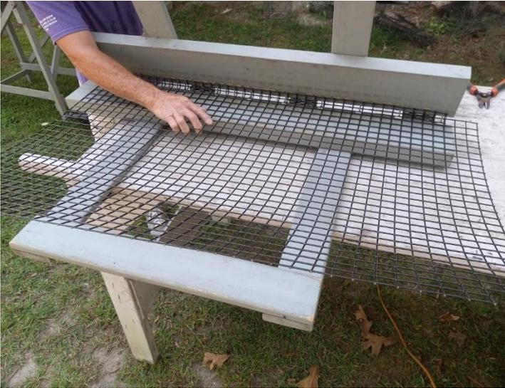
Starting on a long edge, bend the outer 2 rows of mesh into a triangular stiffener, as shown, using ~ 135 degree bends. Repeat on the opposite long edge.
