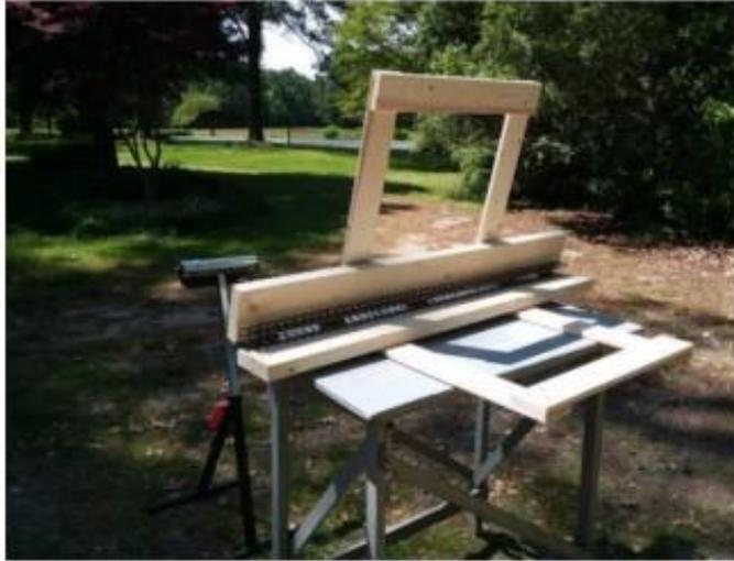
First a  $\sim 3/8$  in. chamfer is cut along each 2x6. This is to make room later for the hinge barrels.
