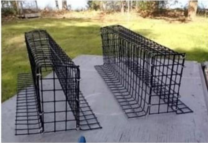
Use a bender and pig rings to make feet. Wire pieces are 21" by 19":: Bend the wire along the 21" edge for each foot, then add the 3" by 6" panels at each end for stiffness. Attach feet to cage with pig rings.
