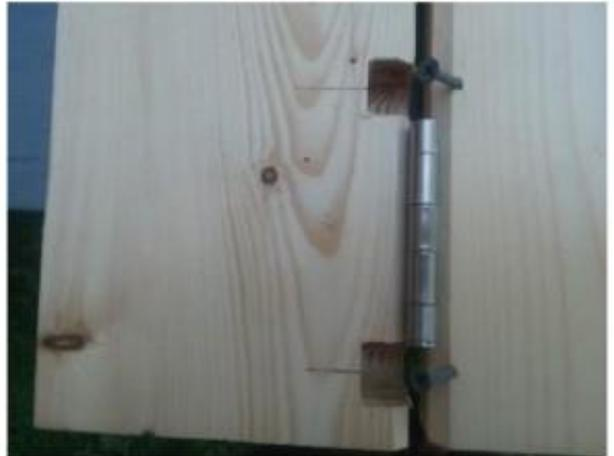
Place 3 inch door hinges between the screws as shown. I like to use 1.25 deck screws rather than the screws that come with the hinges.
