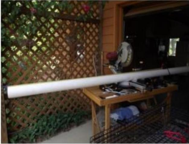
PVC drain or sewer pipe comes in 10 ft. lengths. Cut 2 38" pieces. You will have an extra piece for your next flip float. You can cut with a chop saw, jigsaw, circular saw or hand saw.
