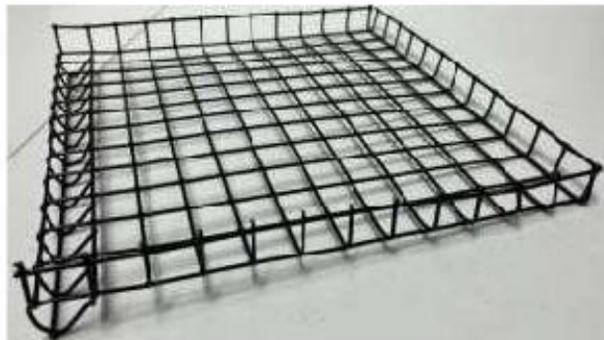
End hatch piece bent and ready for assembly
