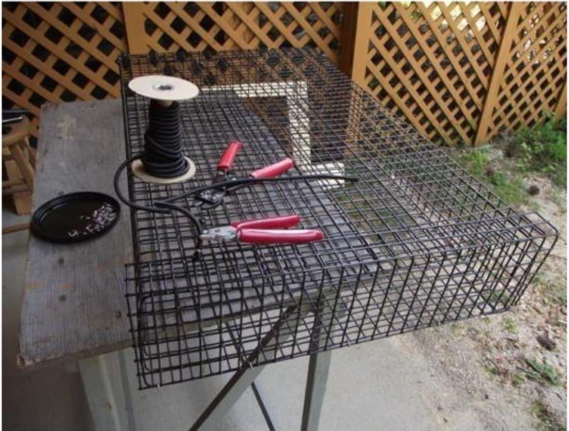
Cut a 23" length of bungee cord. Attach one end as shown with 2 pig rings.
