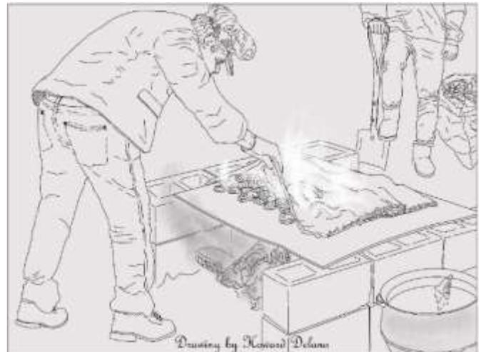
Two low walls about 16 inches high would have to be built from flat sandstone or cinder blocks and located about three feet or a little more apart to contain the fire. A heavy gauge steel plate approximately 36 inches by 48 inches would have to be made ready to pull onto the walls over the hot coals.
